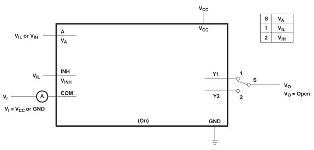
Figure 4. On-State Switch Leakage-Current Test Circuit
